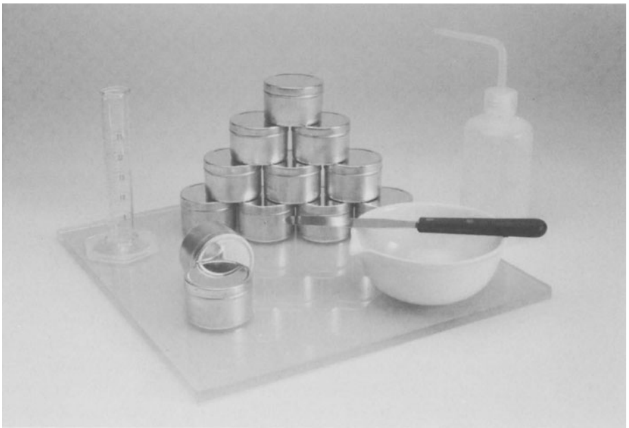
FIGURE 11-3. Plastic limit testing set. [Ref. 4]
