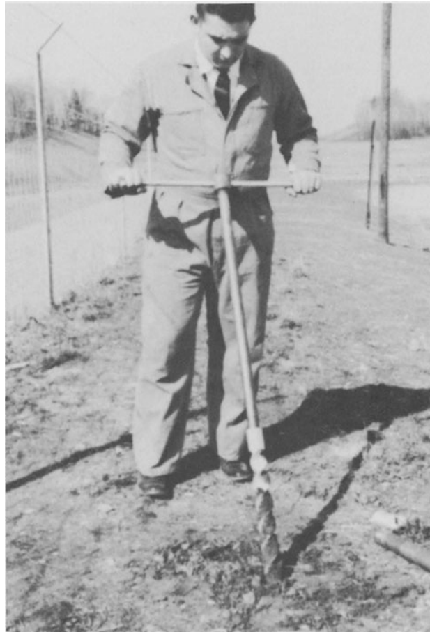
FIGURE 3-1. Ship auger, used in procuring samples of soil by hand. [Ref. 1]
