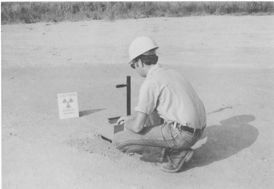
FIGURE 10-9. Soil density using nuclear methods. [Ref. 4]
