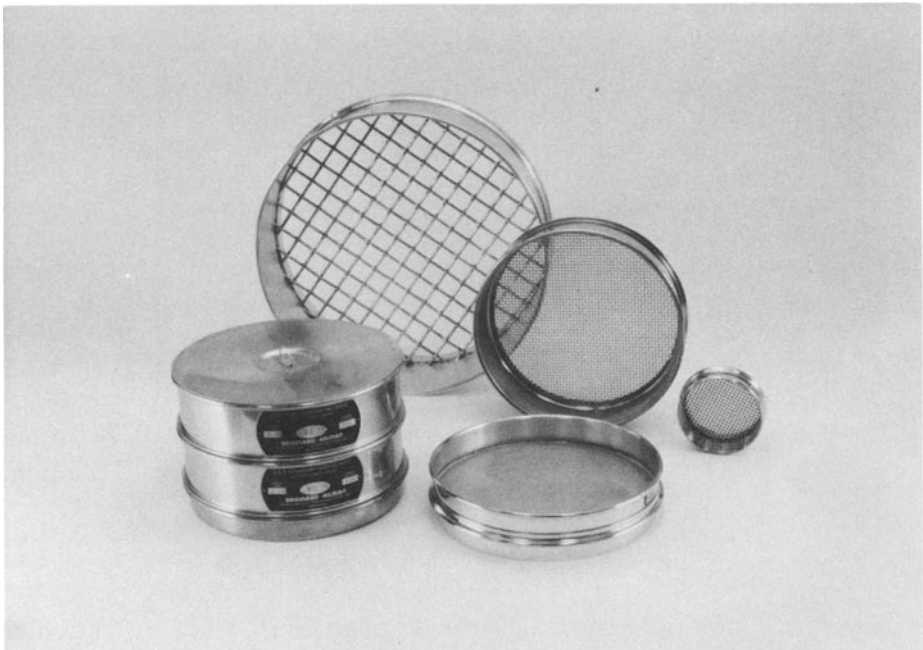
FIGURE 1-1. Standard testing sieves for particle size analysis. [Ref. 4]
