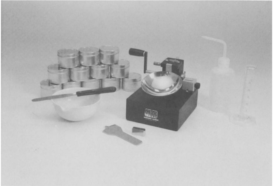
FIGURE 11-2. Liquid limit testing set. [Ref. 4]
