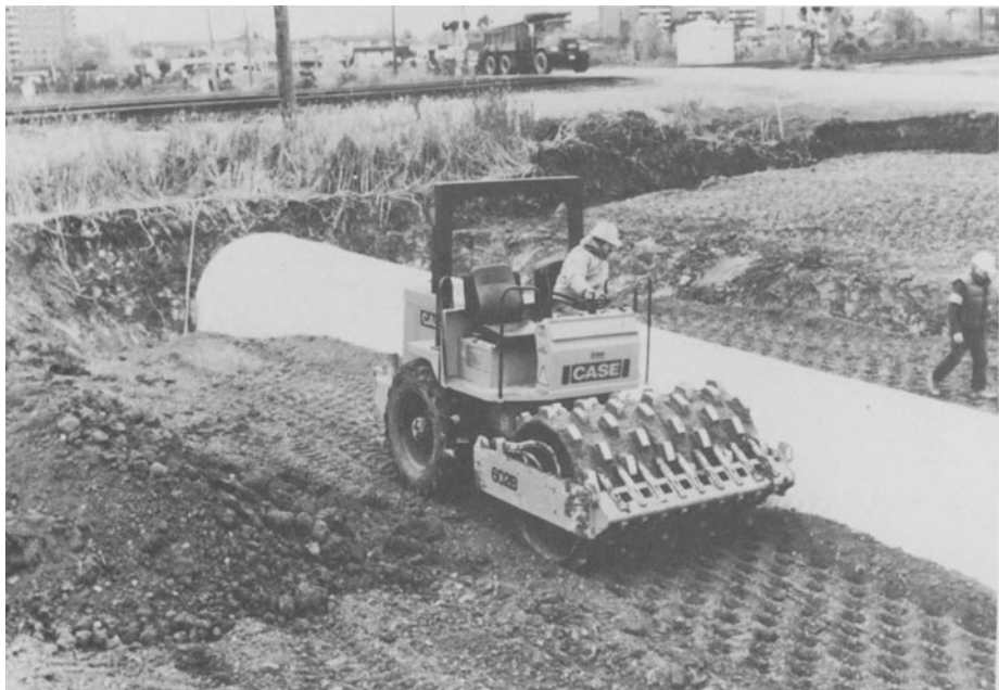
FIGURE 10-3. Different types of machine driven vibratory compactors. (a) smooth drum roller, (b) paddlefoot drum roller. [Ref. 7]
